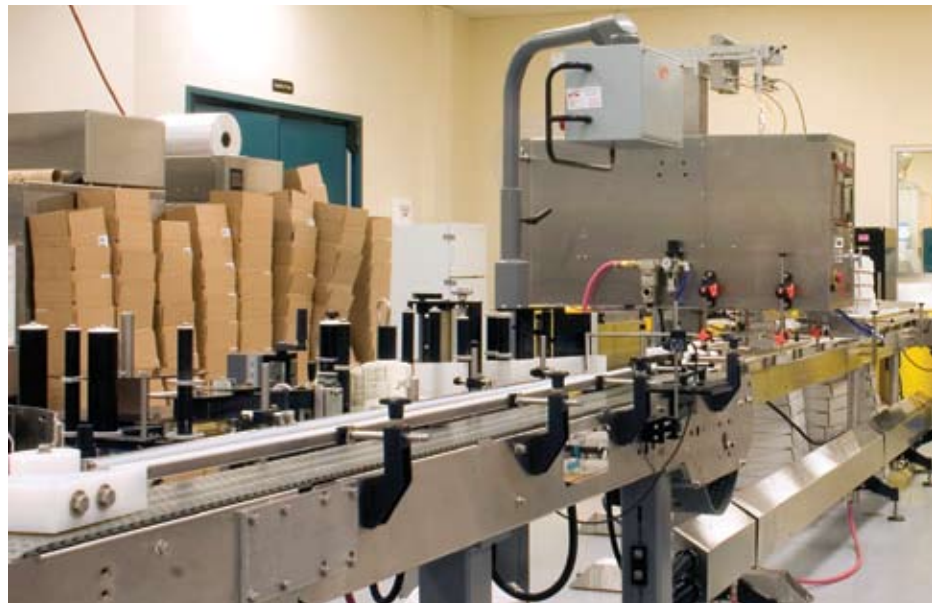
After p-s labeling, supplements are conveyed to a neck banding machine and then through a heat tunnel.
