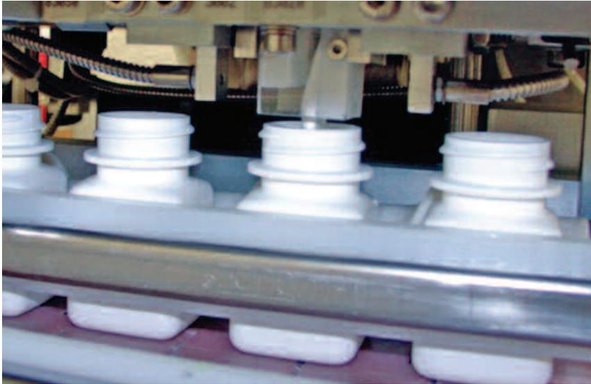
The desiccant feeder drops a single 1-g silica-gel sachet into each bottle, providing sufficient protection against moisture.
