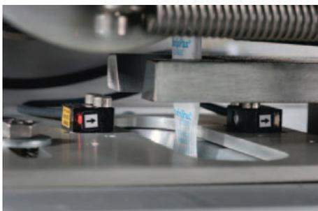
Prior to cutting a StripPax desiccant packet, a servo with an integral encoder on APA equipment ensures exact positioning accuracy.
