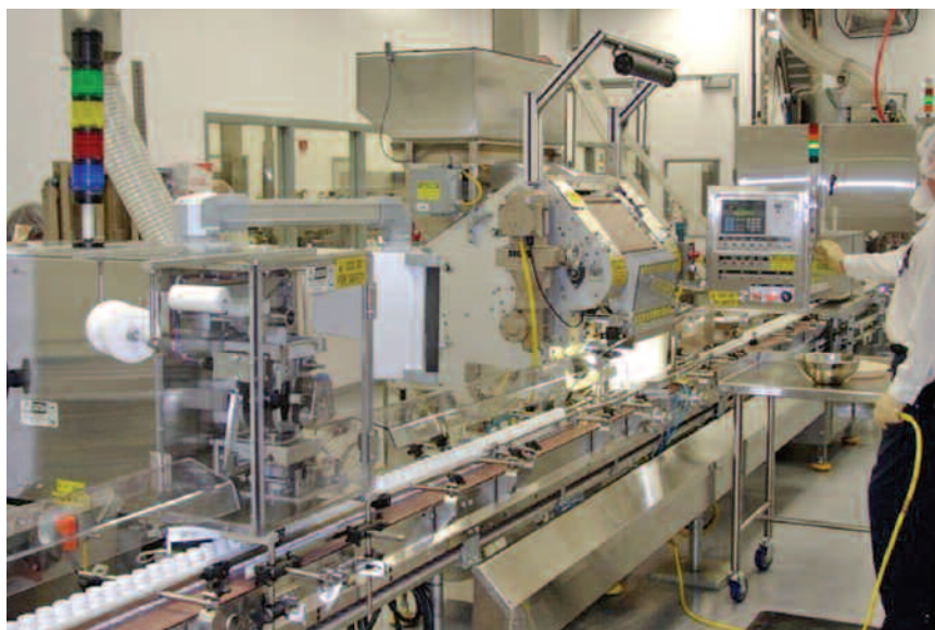
The APA-2000 dispenser, when combined with StripPax sorbent packets, helped increase line speeds from approximately 75 units to almost 95 units per minute.
